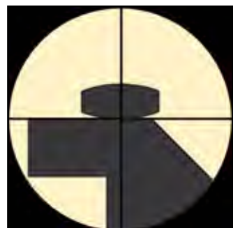
Check tablet profile and flashing
