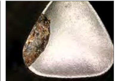
Punch Tip Damage Photo Taken with IN 7951
