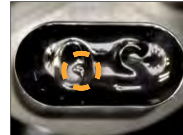
Punch Tip Damage Photo Taken with IN 7951
