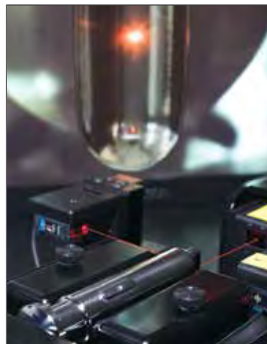
Laser Vision System (LVS) laser focused on punch cup and displayed in real time on monitor
