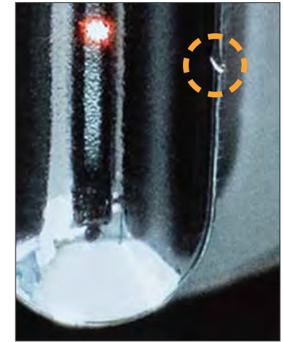
Detect tip damage with the Laser Vision System's camera
